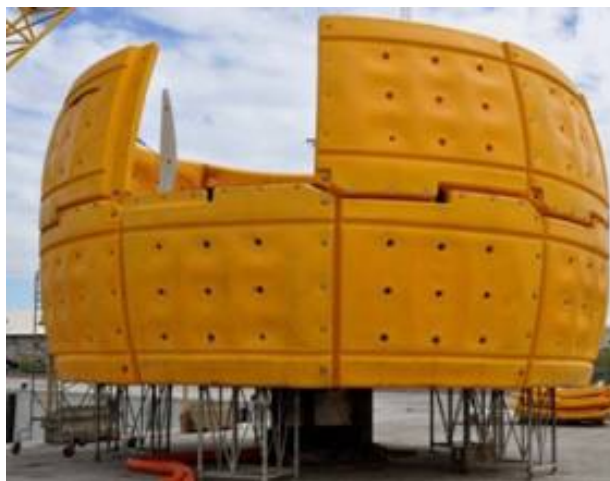
CETO 4 Buoyant Actuator during manufacture
