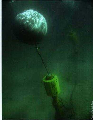
CETO underwater buoys at a Fremantle, WA test site
