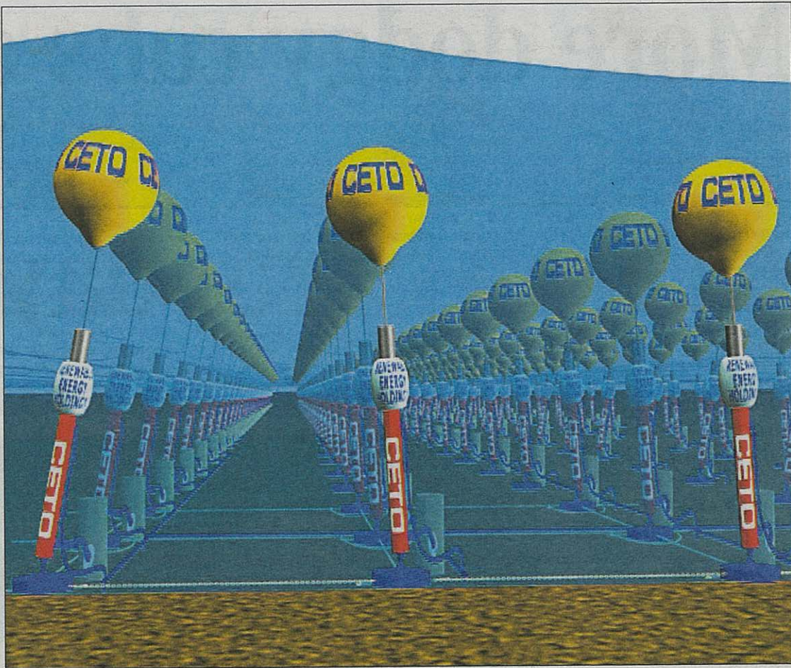
World-first: An artist's impression of a wave farm, consisting of wave energy converter units anchored to the seabed.
